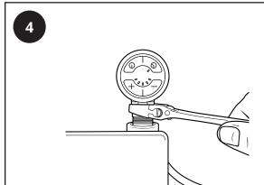
Use an adjustable spanner to tighten the head into the radiator until it is tight and the control faces forward. You can use PTFE tape on the element thread to aid with this. **DO NOT twist the head by hand.**
