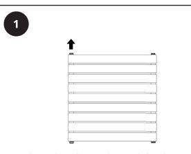
Unbox and stand your radiator with the inlet(s) you will be inserting the element into facing upwards, making sure the unit is sat on a waterproof surface.
