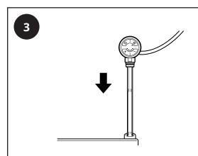
Insert the element into the inlet, some Glycol may spill out of the inlet, this is normal. Clean any spillage with a dry cloth and replace any spilled liquid with water.
