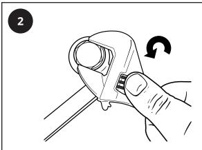
Remove the blanking plug from the inlet you will be fitting the element to by turning the blanking plug anticlockwise.
